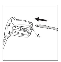
1. Attach the high pressure hose (4) to the spray gun (7). Detach the high pressure hose by pressing the button (A).
