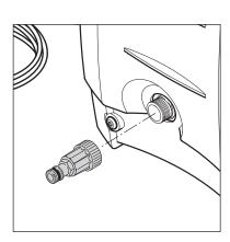
1. Screw the quick coupling tight on to the water inlet (2).
