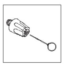
A clogging up in the nozzle causes a pump pressure which is too high. This is why cleaning is required immediately.
