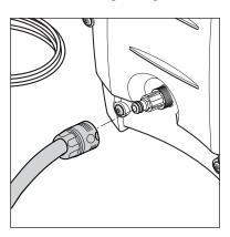
IMPORTANT! Only use water without any impurities. If there is a risk of silt, sand or sediment in the inlet water (i.e. from your own well), an additional filter (106411231) should be mounted.
