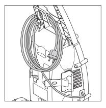
To avoid accidents, the electric cable and the high pressure hose should always be wound up carefully around the handle.
