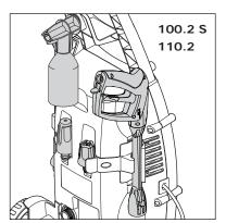
The spray handle, lance and nozzles can be stored on the pressure washer.
