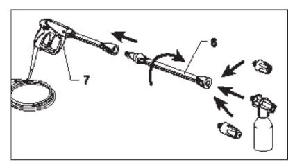
1. Push the spray lance (6) into the spray gun (7) and twist it until the bayonet coupling locks into position.
